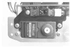
Viewing the servos from the chassis bottom, adjust their positions so that their shafts align as closely as possible. Either center both in their respective cutouts, or push them both toward (not away from) the sensor connector. Just make sure they're the same. Now tighten all eight servo screws.
