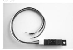
Next, take one of the mounting plates, and thread the wires from one of the cables through the oblong hole. Insert the sensor's alignment pin into the mating mounting plate hole. Secure the sensor to the mounting plate with a screw through the other set of holes and a nut on the back. Repeat for the other sensor, but with the opposite orientation. When finished you will have two mounted sensors that are mirrors of each other:
